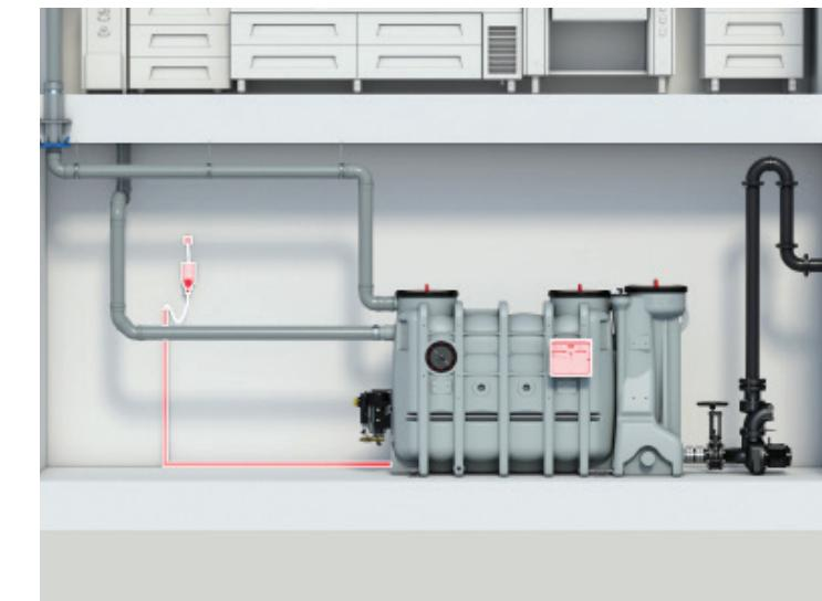
ACO LipuSmart, the solution integrating both grease separator and lifting station includes only one control unit which is mounted integral with the separator ex works. The control unit enables fast and simple function of both applications by operators or installers.
