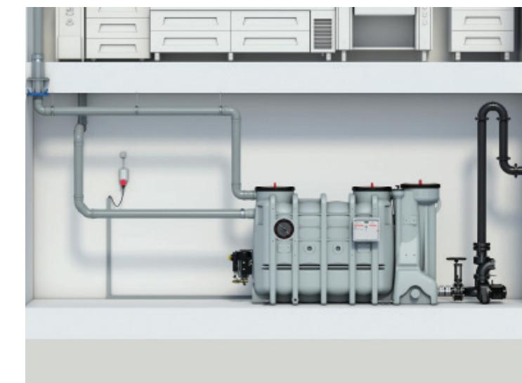
With ACO LipuSmart it is not needed to create pipe connections between separator, sampling unit and lift plant anymore because ex works all components have been connected and checked for tightness.
