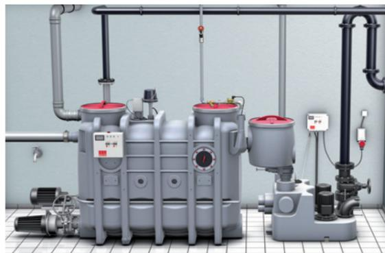
Waste water lifting plants convey waste water above the backflow level into the higher sewage system. EN 12056 stipulates that waste water lifting plants must be used where drainage points are below the backflow level, i.e. for almost all free-standing grease separator plants. Depending on the application scope, ACO offers a choice of different waste water lifting plants that can be installed directly behind the grease separators.
