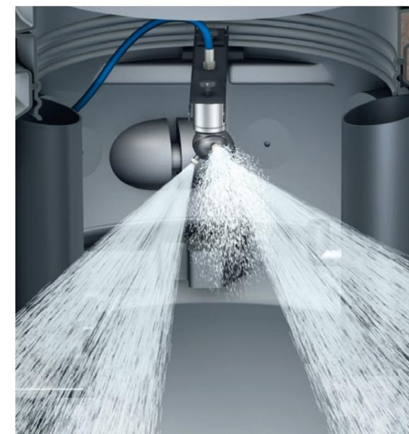
Unpleasant smells produced when disposing of the contents of grease separators are often equated with hygiene deficiencies. In order to prevent this, ACO grease separators are available with optional hydro-mechanic high-pressure inner cleaning. This enables the inside walls of the grease separator to be intensively cleaned, without having to open the covers.
