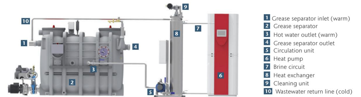
The hot water generated by the catering establishment enters the grease separator (2) through the inlet (1). This wastewater is drawn through the connection sleeve on the grease separator and out of the separator (3) by means of the circulation unit (5). Then the still hot wastewater flow into the heat exchanger (8) where it is cooled down and then it flows back into the grease separator (10).
