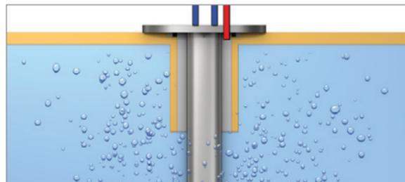
Air is blown into the pilot tube continuously via a compressor. The air bubbles which rise at the end of the pilot tube create a constant motion beneath it, so no media that generate floating surfaces (e.g. residual grease from the separator) are able to set. This guarantees that level measuring equipment works very reliably.
