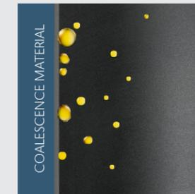
Oil droplets spread over the coalescence material, and additional oil droplets are adsorbed and the oil film continues to grow.
