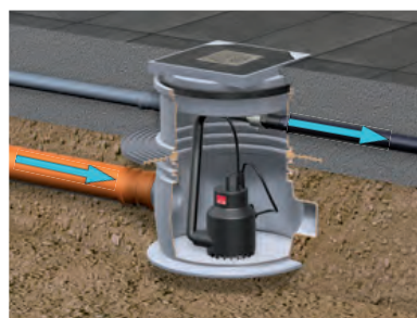
Mono lifting station for grey water
