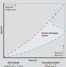
Designed to regulate storm water flows from 2 -100 litres per second, ACO Q-Brake is tailored to the specific performance requirements of the application providing optimum efficiency within the drainage system.
